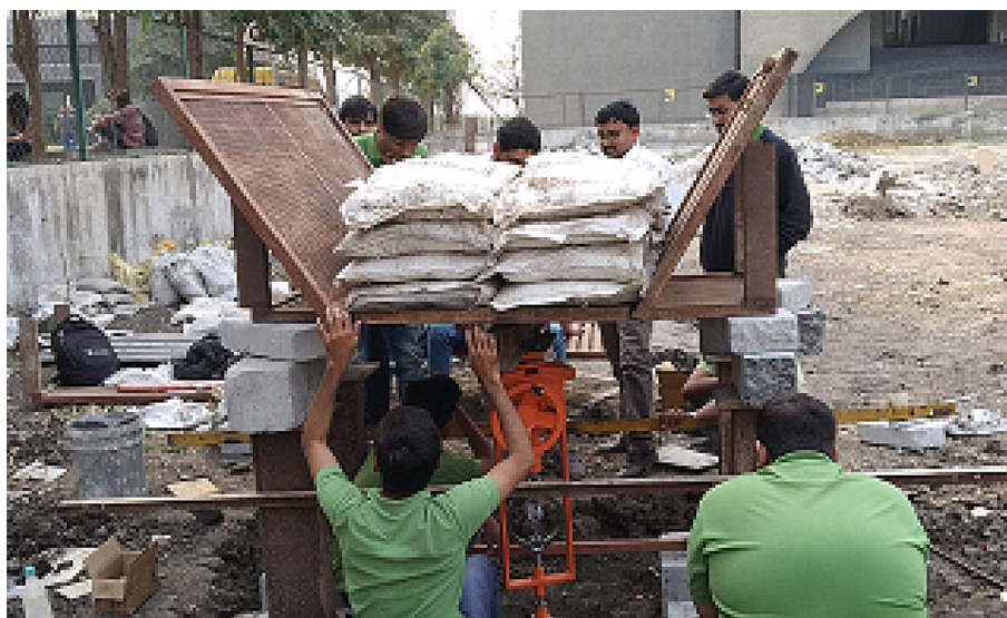
Fig. 9. Plate load test.
