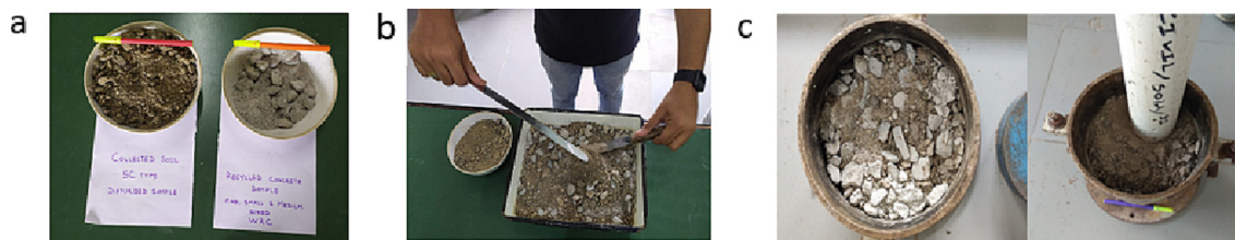
Fig. 2. (a) Material samples;(b) Mixing of samples;(c) CBR test in progresses.
