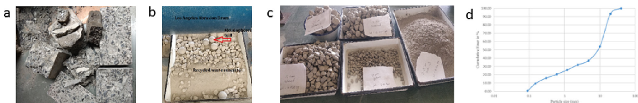
Fig. 1. (a) Demolition waste;(b) Pre-treated waste;(c) Constituents of RWC; (d) Particle Size Distribution curve.
